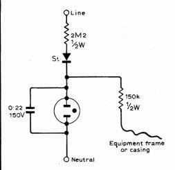
This simple circuit gives a warning if the earth wire is disconnected from the chassis of an instrument. It is particularly useful for oscilloscopes which may be left in a hazardous state when the earth wire is purposely disconnected to avoid hum loops etc.
